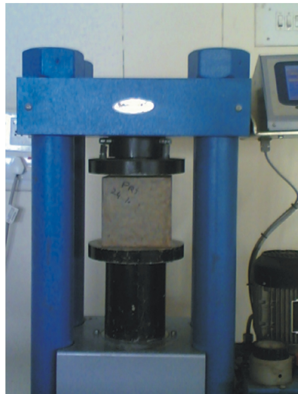
Fig. 2. Testing of specimen in compression testing machine
