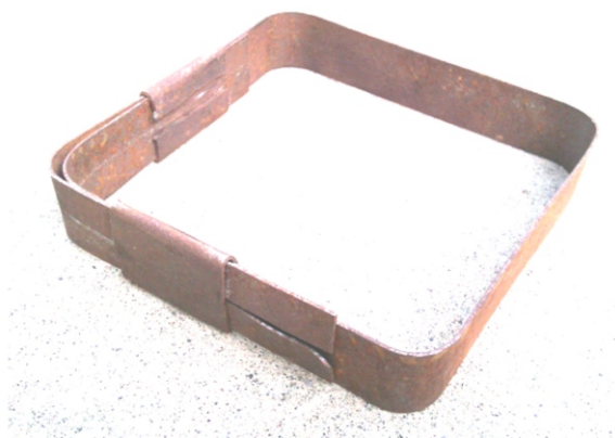
Fig. 3. End anchorage condition of hooked strip
