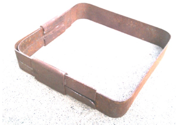
Fig. 3. End anchorage condition of hooked strip
