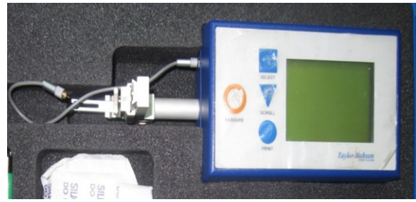
Fig. 5. Profilometer employed for the measurement of surface roughness ( R_a ).
