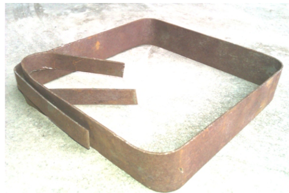
Fig. 4. End anchorage condition of stapled strip
