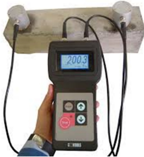
Fig. 1. (a). Ultrasonic Concrete Tester
