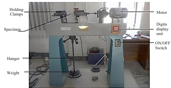
Fig. 5. Fatigue test experimental setup
