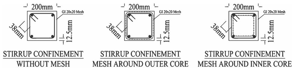
Fig. 1. Structural detailing of specimens
