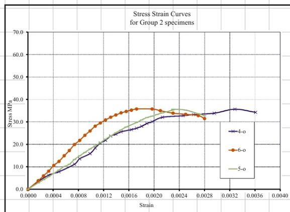
Fig. 9. Stress strain curves for group-2 specimen (Outer core confined by GW Mesh)
