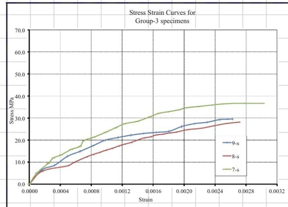
Fig. 10. Stress strain curves for group-3 specimen (No GW Mesh)
