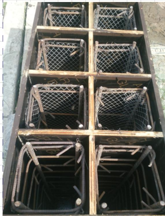
Fig. 3. Specimens placed in form work, ready for pouring
