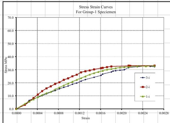
Fig. 8. Stress strain curves for group-1 specimen (Inner core confined by GW Mesh)
