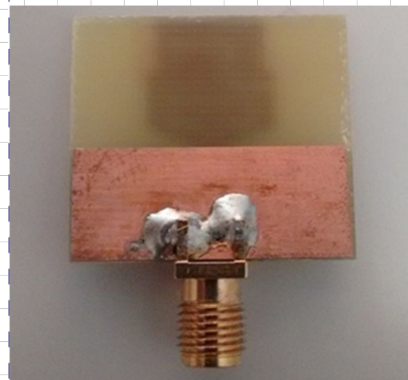
Fig. 7. Fabricated image of proposed antenna with triple stop bands: Front View and Back View
