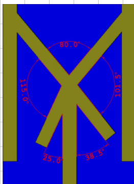
Fig. 3. Angles between arms and feed line of m-shape patch
