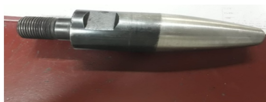
Fig 2: Forging Punch after Heat Treatment
