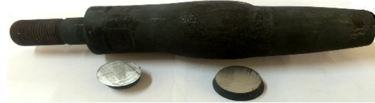
Fig 7: Deformed sample of AISI H13 tool steel
