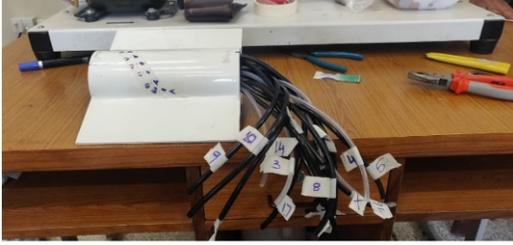
Fig. 4: Visuals of pressure taps on circular cylinder with attached rigid bilateral splitter plates
