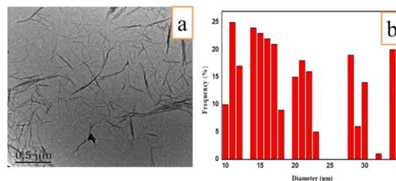
Fig. 3. (a) TEM image for the cellulose nano fibers prepared with 2 h TEMPO oxidation (b) Diameter-frequency histograms of cellulose nano-crystals
