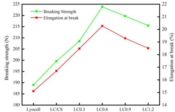
Fig. 5. Tensile strength and elongation at break of pristine and modified Lyocell fabrics with constant chitosan and varied fractions of CNC
