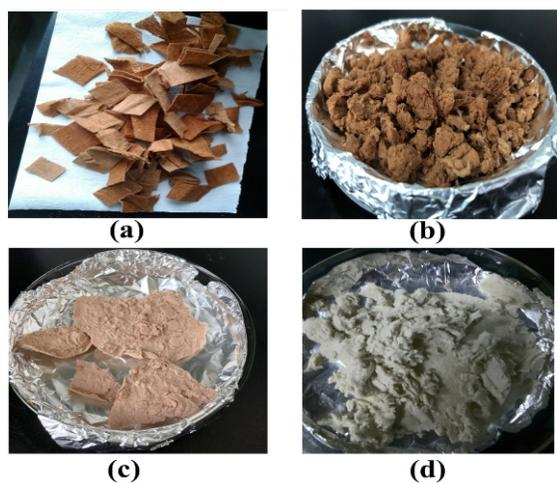
Fig. 1. Photographs of bark cut pieces: (a) chopping of the samples (b) sample washing to remove impurities (c) alkali-treated samples, and (d) cellulose fibers after bleaching
