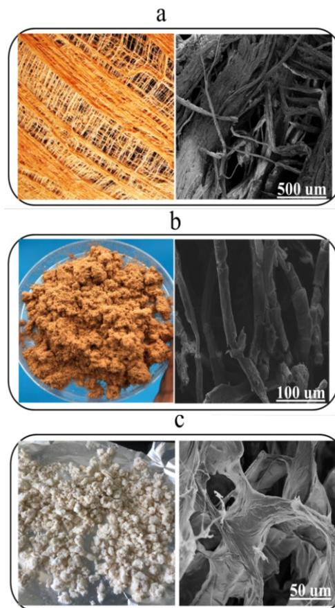
Fig. 2. Scanning Electron Micrographs at various stages of *Ficus natalensis* bark-cloth during cellulose extraction process (a) bark-cloth without any treatment, (b) after converting into powder form (c) Freeze dried cellulose nano-crystals.
