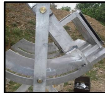
Fig. 11 Target “D” mounted with 12.7 mm air gap
