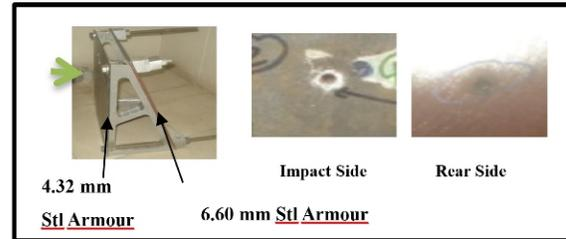
Fig. 18 Target “Q” configuration, impact side and exit side
