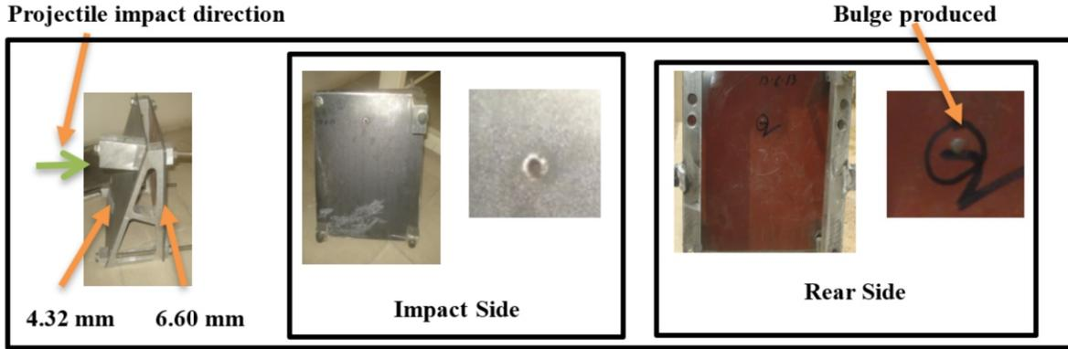
Fig. 19 Target “F” with projectile indentations
