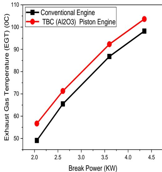
Fig. 10: Discrepancy of EGT of TBC engine and conventional engine under diverse break powers.
