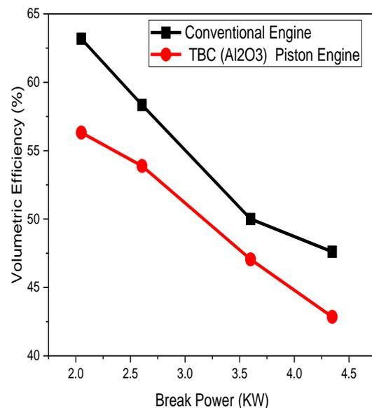
Fig. 9: Discrepancy of VE of TBC engine and conventional engine under diverse break powers.
