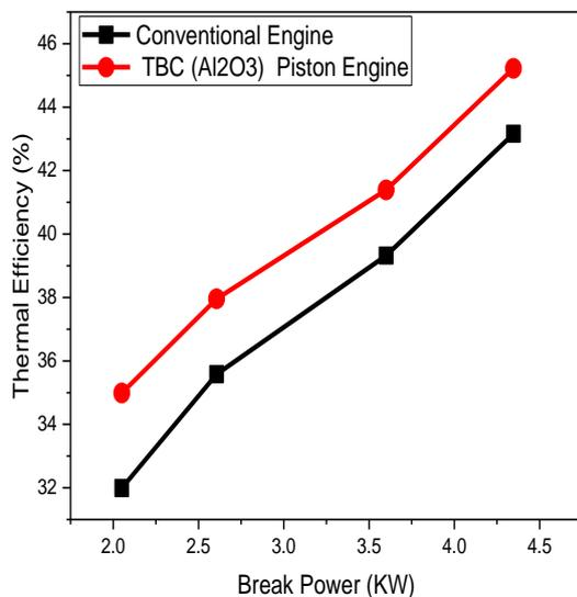
Fig. 6: Discrepancy of TE of TBC Conventional engine under diverse break powers
