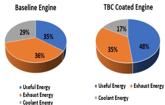
Fig. 1: Energy balance of the conventional and ceramic TBC engines.
