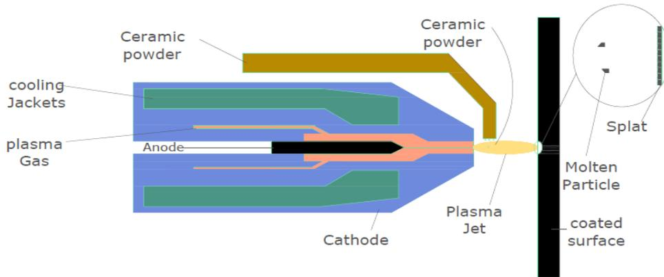
Fig. 2: Illustration of plasma spray technique (PST).
