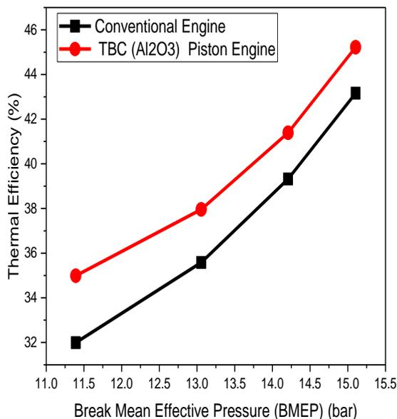
Fig. 8: Discrepancy of TE of TBC engine and conventional engine under diverse BMEP.
