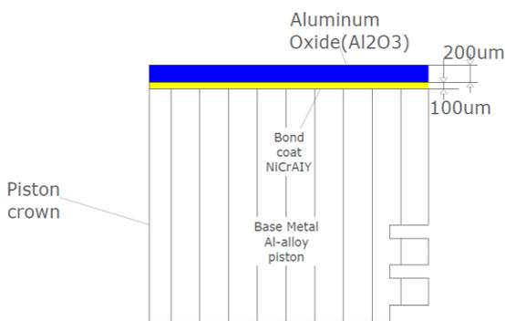
Fig. 4: Binder and coated material thickness on the piston crown.
