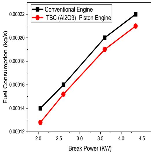
Fig. 7: Discrepancy of fuel consumption of TBC engine and conventional engine under diverse break powers.
