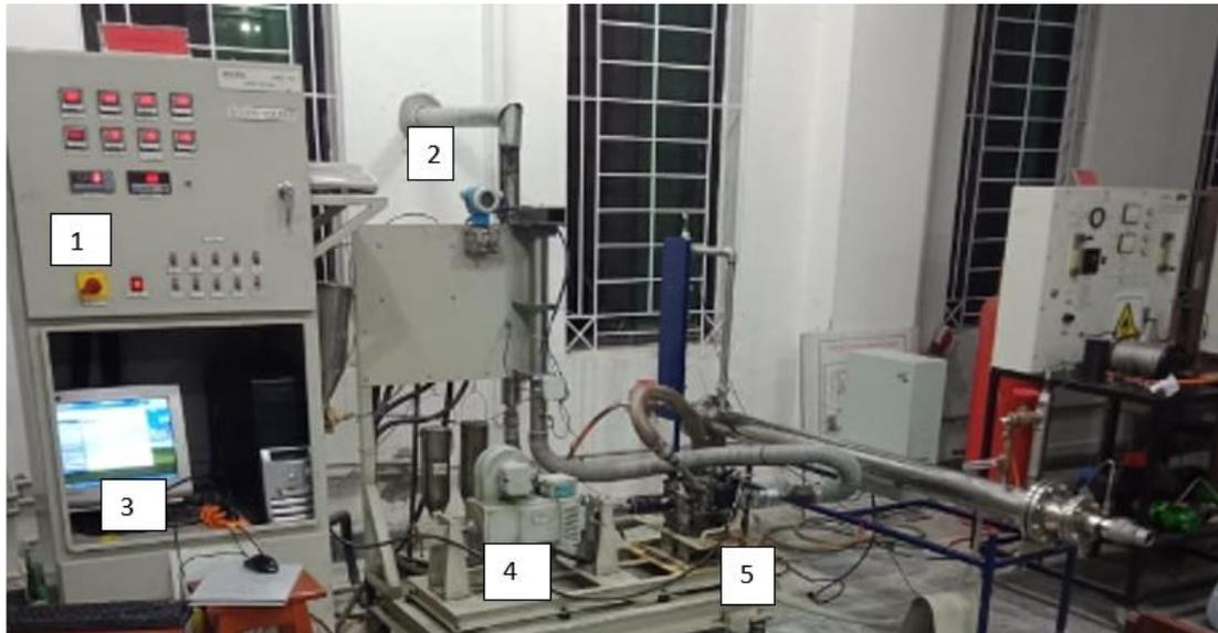
Fig. 5: Engine Test Bed
