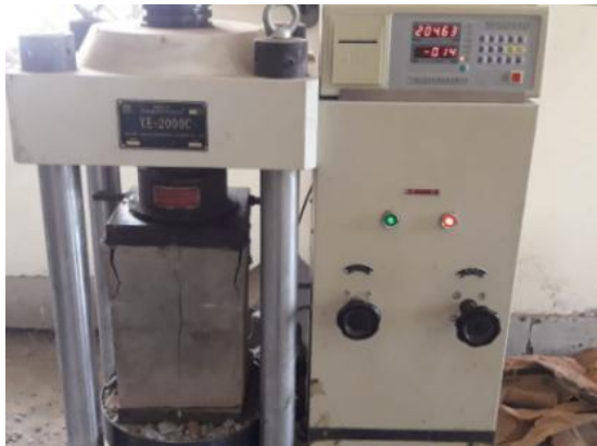
Fig. 14 Compressive Strength testing of fire untouched prism
