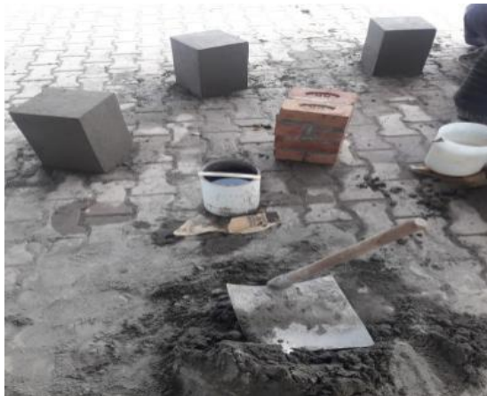
Fig. 8 Construction of masonry prism
