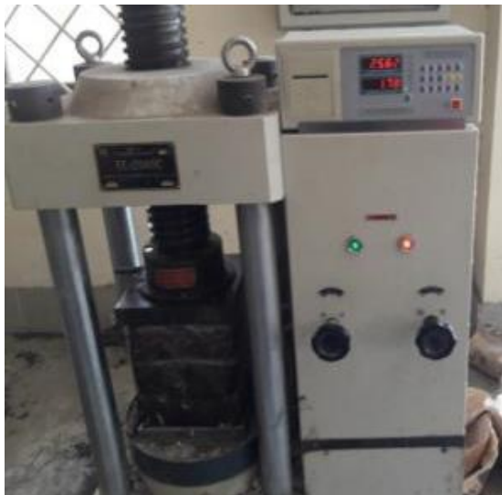
Fig.15 Compressive Strength test of prism without PVC wall panel
