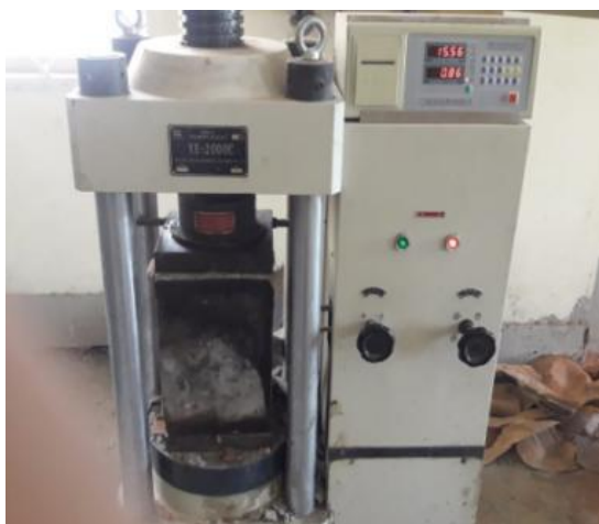
Fig. 16 Compressive Strength testing of prism without PVC wall panel 2
