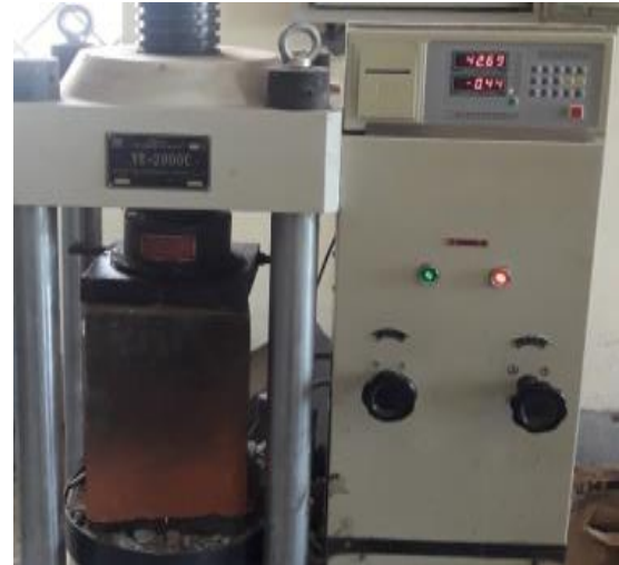
Fig.17 Compressive Strength testing of the prism with PVC wall panel
