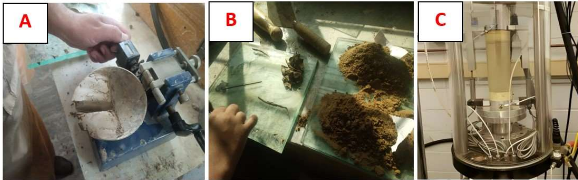
Figure 1:(a) Liquid Limit Testing, (b) Plastic Limit Testing, (c) Triaxial Testing
