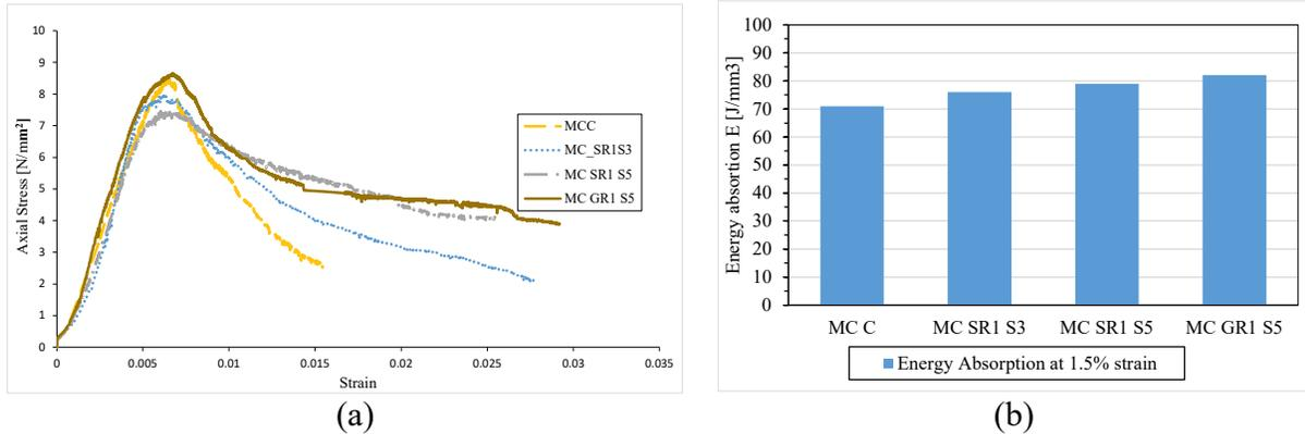
Figure 5: (a) Stress-Strain curves of specimens (b) Energy absorption bar charts of specimens
