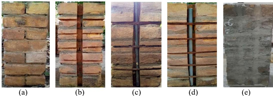
Figure 3: Specimens preparation (a) stage 1 (casting) (b) Stage 2 (grooving) (c & d) stage 3 (specimen retrofitting) (e) stage 4 (groove backfilling)
