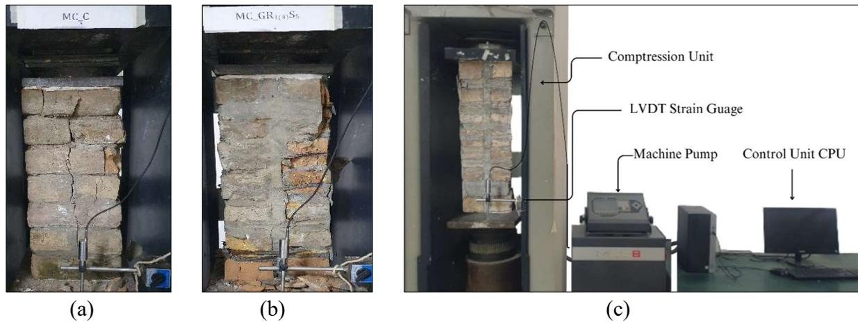
Figure 4: (a) control specimen (b) Retrofitted specimen (c) Experimental testing setup
