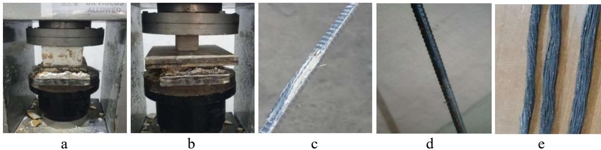
Figure 1: Material (a) Brick Sample Testing (b) Mortar Cube Testing (c) Tested GFRP bar (d) steel reinforcement (e) small diameter steel bars
