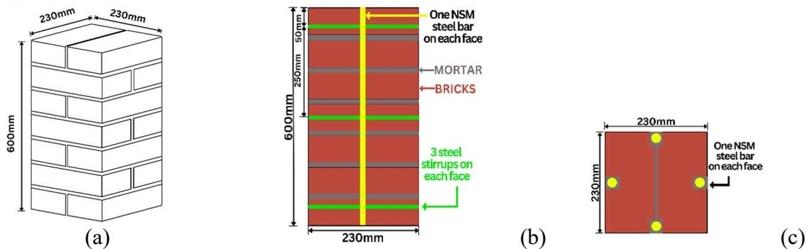
Figure 2: Sample Details (a) Control specimen (b) Strengthened specimen side view (c) Top view
