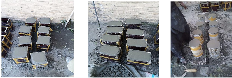
Figure 2 Casting of samples
