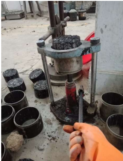
Figure 2: Demolding of Marshall Sample
