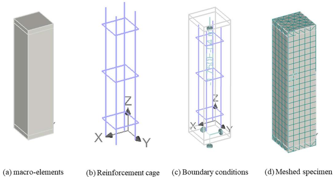
Figure 6 Details of FE model
