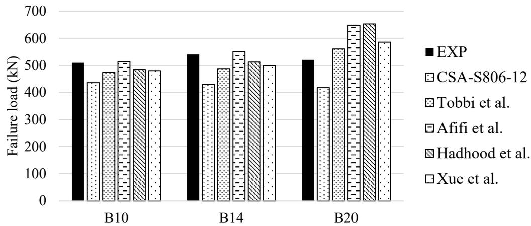
Figure 5: Comparison between predicted and experimental load-carrying capacities of BFRP RC columns
