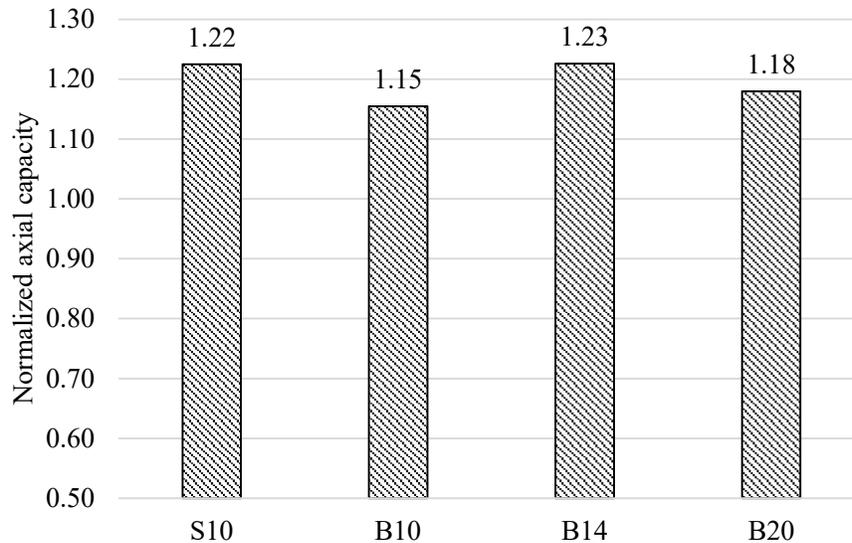
*Figure 3 Axial load-carrying capacities of concentrically loaded columns normalized to plain concrete specimen*
