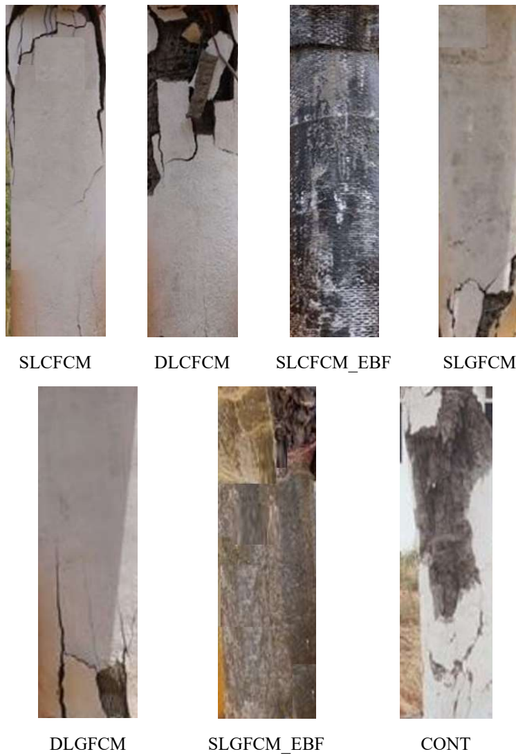
Figure 6: Failure modes of the specimens
