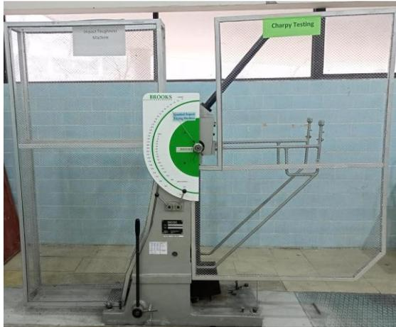
Figure 4. Charpy Testing Machine
