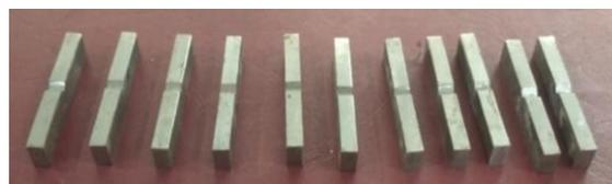
Figure 3. Charpy V-notch specimens
