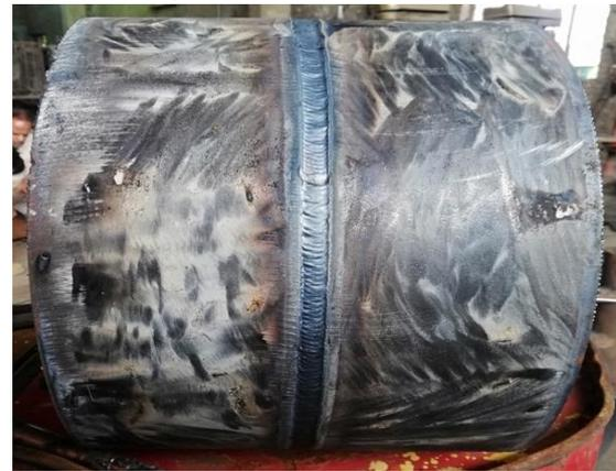
Figure 1. Welded pipe of API x60
