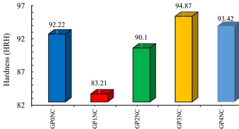
Figure 3: HRD values of HFPG mix for different extents of calcium carbonate
