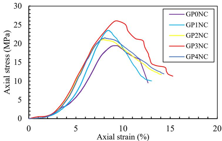
Figure 1: Effect of calcium carbonate concentration on compressive stress-strain efficiency of HFGP mix
