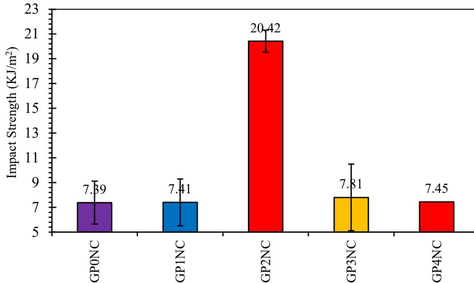
Figure 4: The HFGP blend's IST values at different concentrations of calcium carbonate
