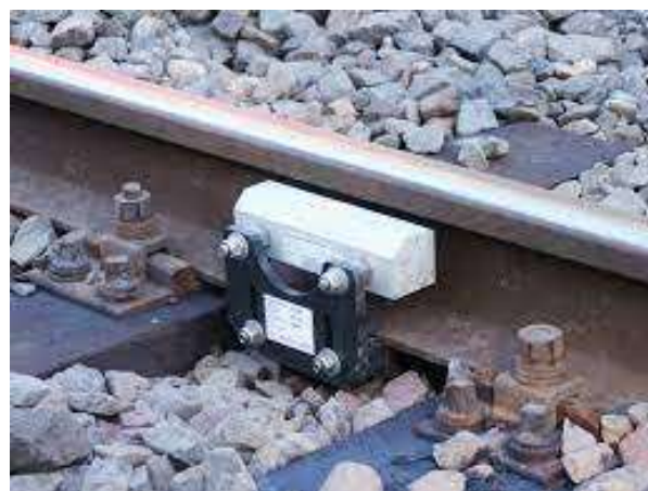
Figure 3: Axle Counter which Counts number of wheels moving over it
