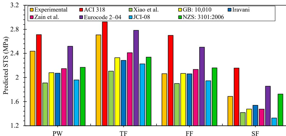
Figure 5: Comparison of STS forecasts for RGC blends using various equations
