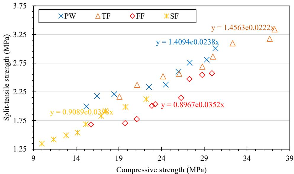
Figure 4: Forecasts for the CS and STS of RGC blends using various codes
