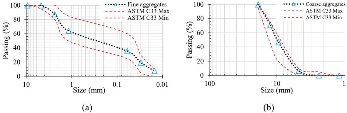
Figure 1: Granulometry (a) sand (b) RCA
