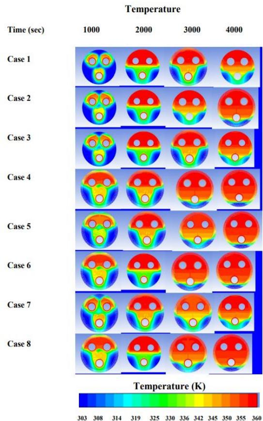
Figure 19 Temperature of Melting Fractions
