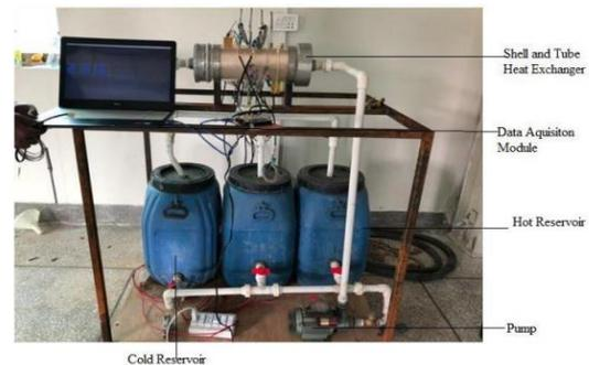
Figure 7. Experimental Setup
