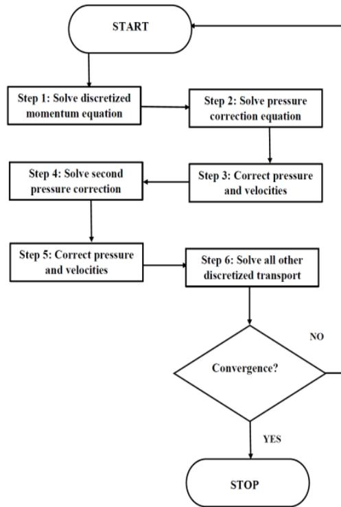
Figure 3. PISO Algorithm Flowchart
