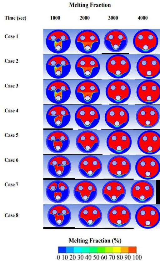
Figure 14 PCM Melting Fraction Contours
