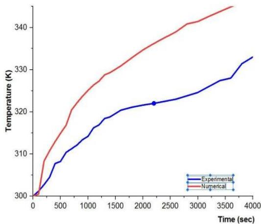
Figure 18. Melting Temperature Comparison of Numerical and Experimental Results
