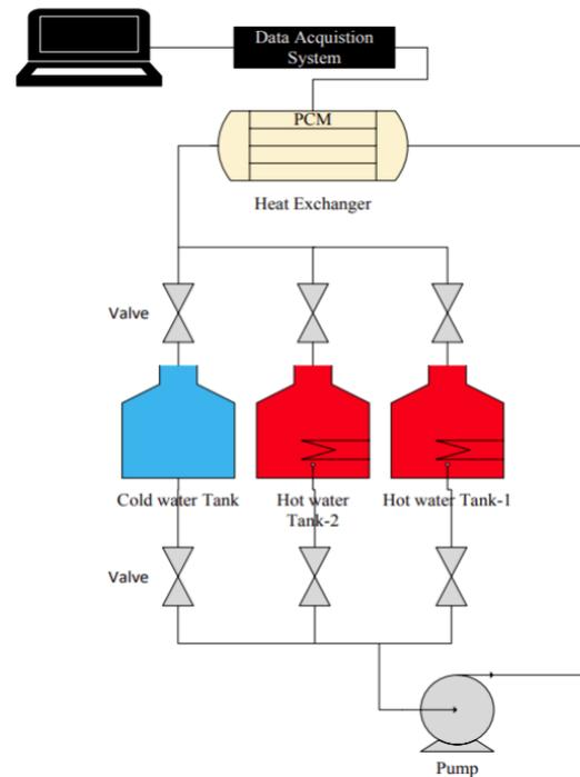
Figure 2. Schematic Diagram of Prototype
