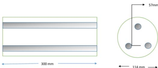
Figure 5 Selected tube orientation for Shell and tube Heat Exchanger
