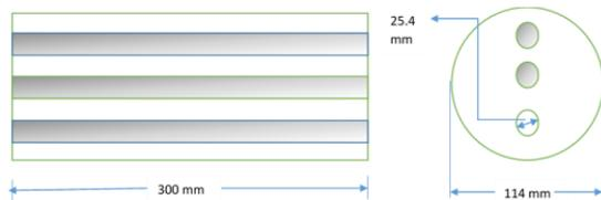
Figure 4. Shell and tube heat exchanger model used for simulation
