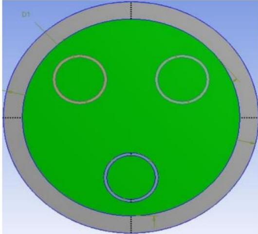
Figure 9. Cross-sectional view of Heat Exchanger with tubes and shell, filled with PCM
