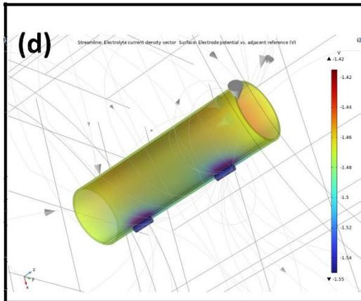
Figure 9: Cathodic Protection Results of Pipeline using Magnesium Sacrificial Anode showing (a) Electrolyte Potential, (b) Electrolyte Current Density, (c) Electrode Potential vs Ag/AgCl Reference Electrode, and (d) Transparent View of Electrode Potential vs Ag/AgCl Reference Electrode
