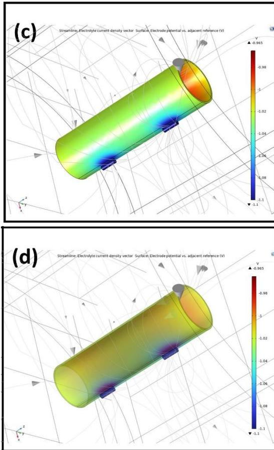
Figure 7: Cathodic Protection Results of Pipeline using Aluminium Sacrificial Anode showing (a) Electrolyte Potential, (b) Electrolyte Current Density, (c) Electrode Potential vs Ag/AgCl Reference Electrode, and (d) Transparent View of Electrode Potential vs Ag/AgCl Reference Electrode
