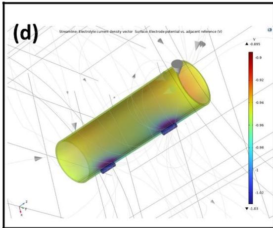
Figure 8: Cathodic Protection Results of Pipeline using Zinc Sacrificial Anode showing (a) Electrolyte Potential, (b) Electrolyte Current Density, (c) Electrode Potential vs Ag/AgCl Reference Electrode, and (d) Transparent View of Electrode Potential vs Ag/AgCl Reference Electrode
