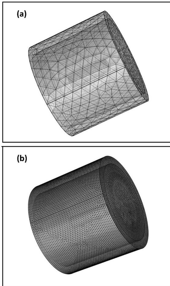
Figure 6: Cathodic Protection Model with (a) Coarse Mesh and (b) Fine Mesh
