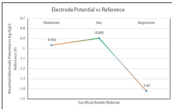
Figure 10: Comparison of Electrode Potential vs Ag/AgCl Reference
