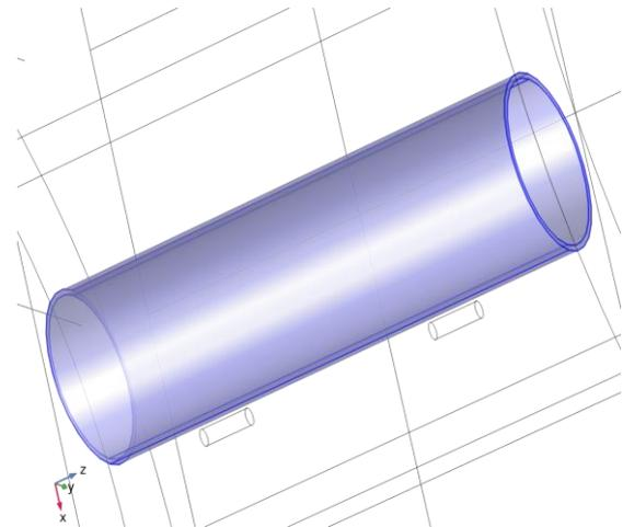
Figure 5: Selected Surface to be Cathodically Protected
