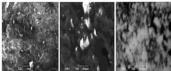
Figure. 2 SEM images of piston crown fueled by DF, DF95WCO5 and DF65WCO20Pe15.
