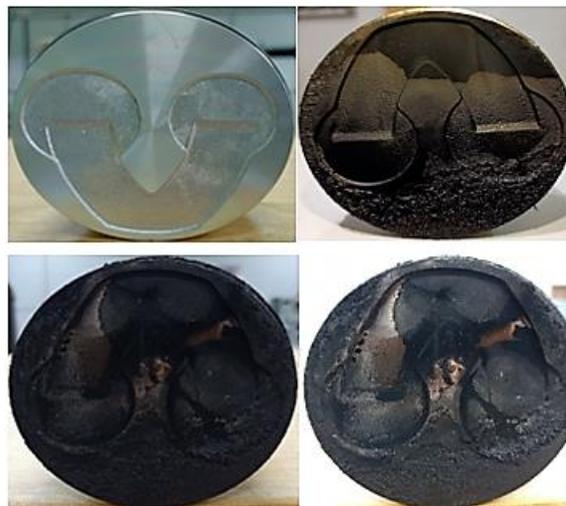
Figure.1 Visual inspection of engine piston during endurance tests.
