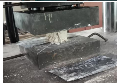
Figure 7: Universal Testing Machine (Max Load 250 KN) for Compressive Strength Testing
