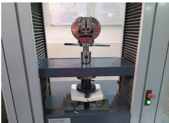
Figure 8: Universal Testing Machine (Max. Load 30 KN) for Flexural Strength Testing
