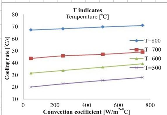
Fig. 10. Cooling rates at different convective boundaries
