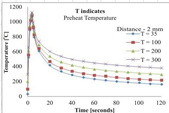
Fig. 7. Effect of metal preheat on temperature profiles
