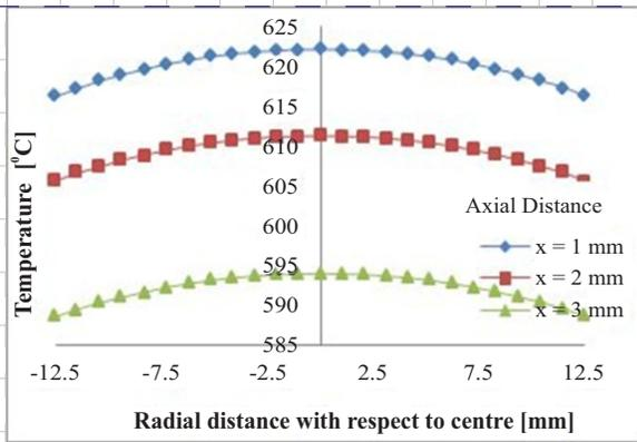
Fig. 9. Temperature profile across bar diameter at various axial distances from center
