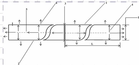
Fig. 1. Heat transfer mode in flash butt welding
