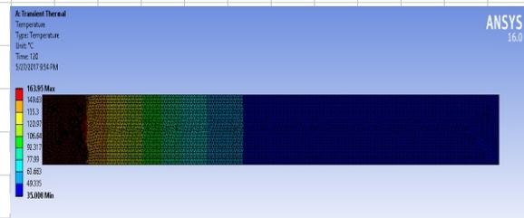
Fig. 3. Temperature field along the bar at 120 seconds
