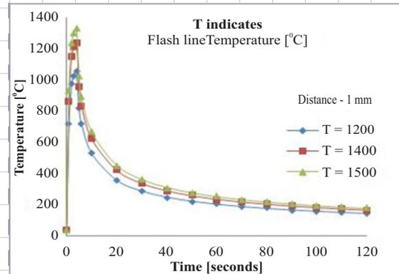
Fig. 8. Effect of flash temperature on temperature profiles
