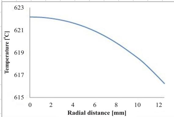
Fig. 6. Peak temperatures variations with radial distance
