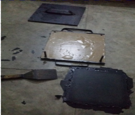
(b) After curing of Kevlar/epoxy with rubber sample Fig. 3.
