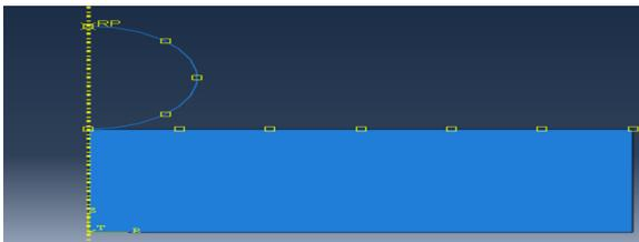
Fig. 3. Indenter and a specimen contact model in Abaqus
