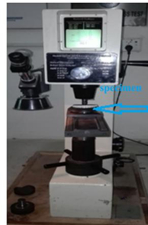
Fig. 1. Hardness Testing Machine
