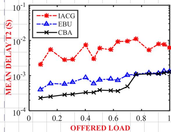
Fig. 5. Mean upstream delay of T2 TCONTs
