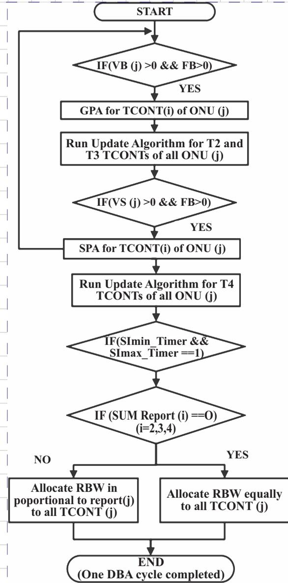
Fig. 2. Flow chart showing CBA DBA Algorithm
