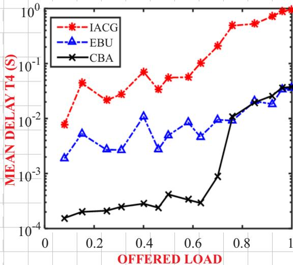
Fig. 7. Mean upstream delay of T4 TCONTs
