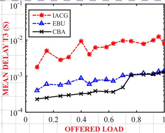
Fig. 6. Mean upstream delay of T3 TCONTs
