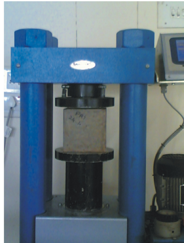
Fig. 2. Testing of specimen in compression testing machine
