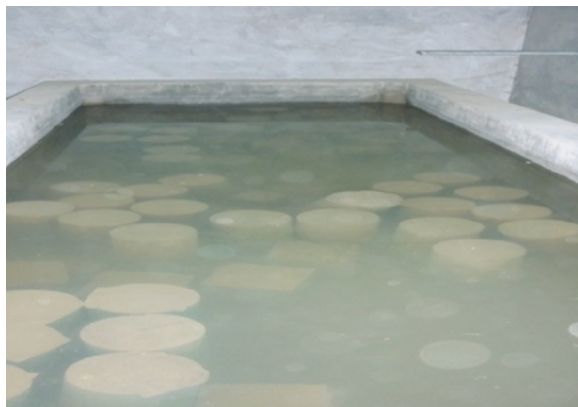
Fig. 1. Curing pond for specimens
