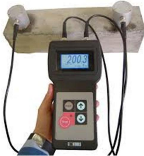
Fig. 1. (a). Ultrasonic Concrete Tester
