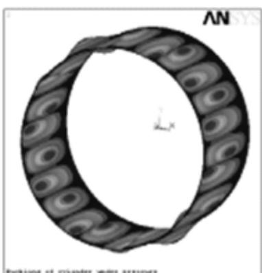
Figure 10: 1st mode shape (Pressure)
