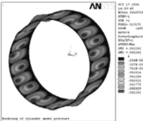
Figure 10: 1st mode shape (Pressure)
