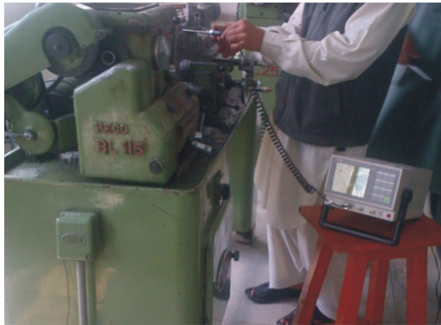
Figure 2 : Experimentation and readings with vibration meter
